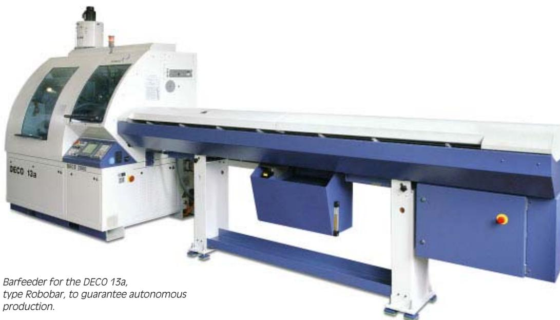
Barfeeder for the DECO 13a, type Robobar, to guarantee autonomous production.
