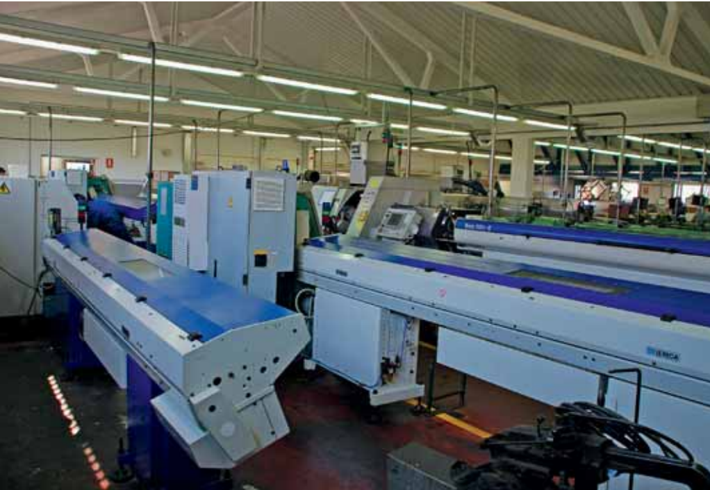
The company's installations, where they combine CNC technology and still very precise cam-type machines.
