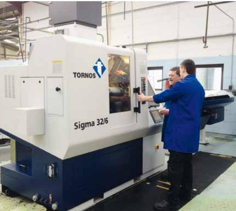
the 7.5 kw spindle power on main and sub spindle that is beyond many fixed head machines was also a major selling point.
