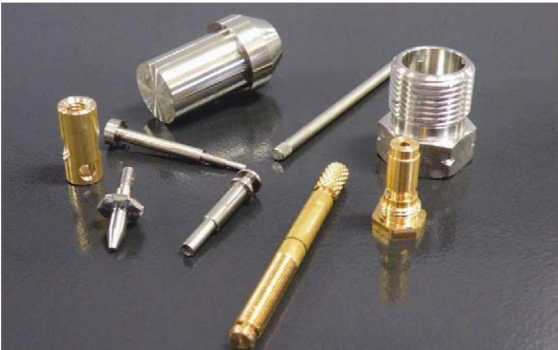
alone have seen parts transferred from the larger machines with a cycle time reduction from 40 to 20 seconds. Another part, a stainless steel pin for specialised shelving applications was drilled, tapped and turned externally and at both ends in 60 seconds, a 15% saving from the larger machines."
