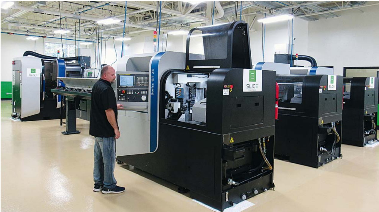
Brad Fowler, Manufacturing Technologist at Slice Mfg. Studios - wide view of 3 Swiss GT 26 machines.
